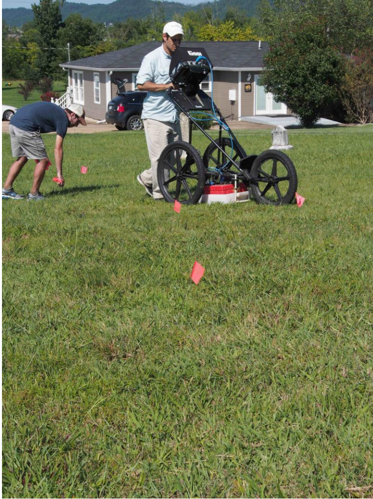
Figure 1. Photograph of Anderson Cemetery survey showing GPR unit and marking flags.
